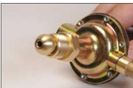
4. Hexagonal nut POL connection CH 25 0,880" 14 NGO Male left
