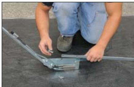
2. Hook the pressure seam roller with lateral handle to the lap torch and fix it with a bolt and wing nut
