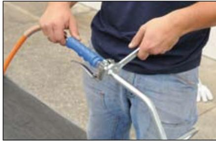
2. Tighten the lap torch nut with a 22 mm spanner
