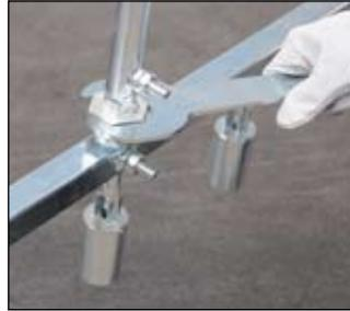
2. Tighten the handle with the 46 mm spanner
