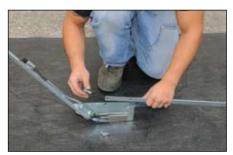
2. Hook the pressure seam roller with lateral handle to the lap torch and fix it with a bolt and wing nut
