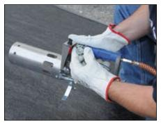
1. Fully open the hot air roofing burner main valve and, at the same time, light the flame by pressing the piezoelectric ignition to start up the burner
