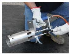
**2.** Connect the compressed air pipe to the hose nozzle of the compressed air device on the hot air roofing burner
