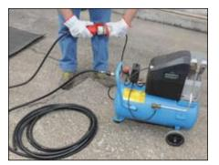
1. Connect an air compressor equipped with a pipe for compressed air to the network current
