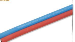
Blue-red coupled rubber hose for oxygen/gas Ø 5 x 12 mm. 20 bar according to EN559
